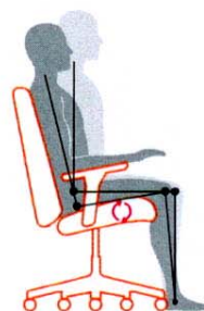
Seats with a synchronic mechanism
